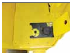
Diesel fuel cap easy access on operator floor
