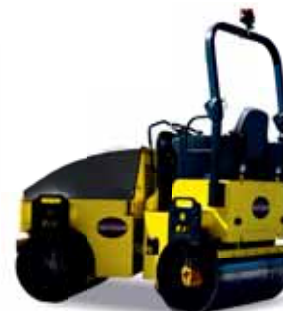
Rotating warning light and serial ROPS protection
