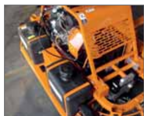
Two water tanks
