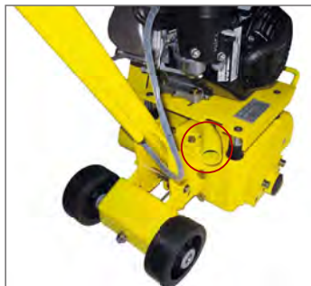
Outlet for dust collector
