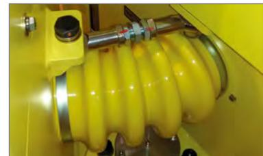
Double articulation with lubrication points 'Pac-Pivot' (patented)
