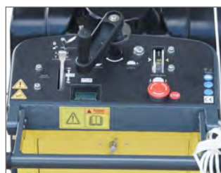
Advanced control panel with hour meter
