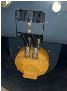
Lubrication point on each cylinder and Poclair drive motors
