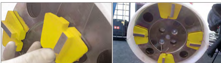
Diamond segments easy to change, without any tools needed
