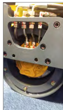
Two hydraulic Poclair pumps
