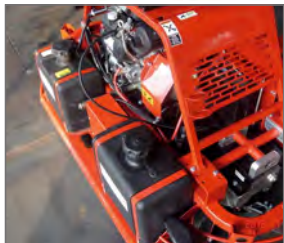
Two water tanks
