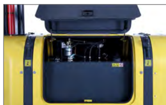
Service hood, carbon components to reduce weight
