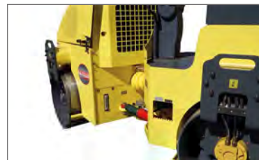
Double articulation with lubrication points 'Pac-Pivot' (patented)
