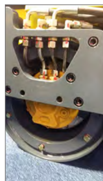
Two hydraulic Poclair pumps
