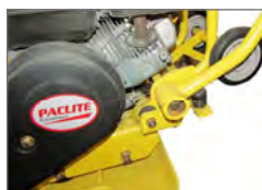
System to reduce HAV (Hand-arm Vibration)
