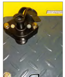
Anti-theft central locking mechanism
