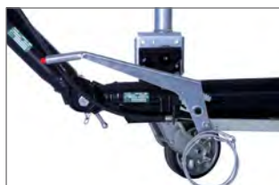
Hand brake and height adjustment
