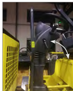
Adjustable ergonomic steering wheel
