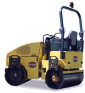
Rotating warning light and serial ROPS protection
