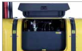
Service hood, carbon components to reduce weight
