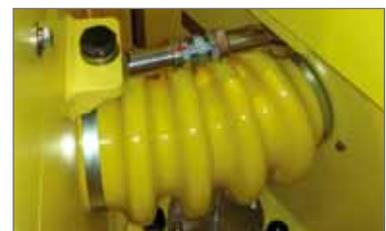
Double articulation with lubrication points 'Pac-Pivot' (patented)
