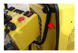
Solution: In this present prototype machine we cannot do much on this problem. This happened because of slight misalignment while welding the structure; we have made further changes to avoid this problem in future.
