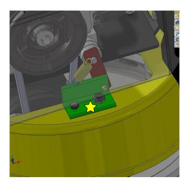
Check the Orientation of the part.. Rear face should be parallel to the cut in the base.
