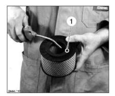
Use compressed air to blow through the filter cartridge from the inside outwards, until further dirt emerges
