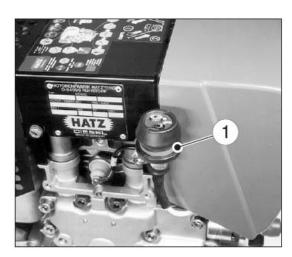
If the rubber bellow shrinks and covers the green area (Point 1), it indicates that air cleaner system should be serviced.
