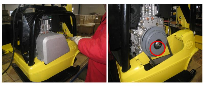
2°) Remove the frame of the base:
