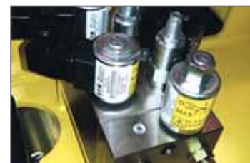
Hydraulic system line assembled, improves security and full power on cylinders.
