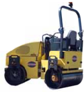
Rotating warning light and serial ROPS protection
