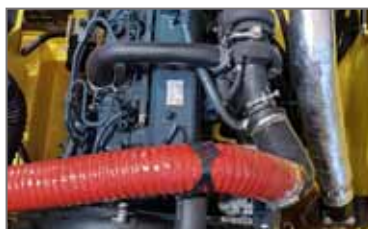
Turbo engine 44 hp to amplify extra power
