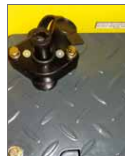
Anti-theft central locking mechanism
