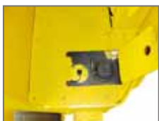
Diesel fuel cap easy access on operator floor
