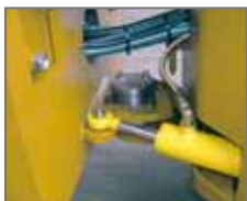
Unique pivot articulation with grease point
