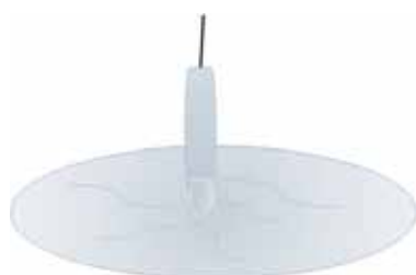
The influence of Zone is determined by the diameter of vibrator head.
