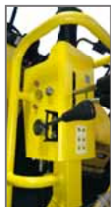
Control panel with double amplitude
