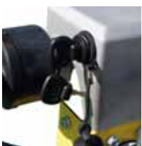
Handle with integrated electric starter box
