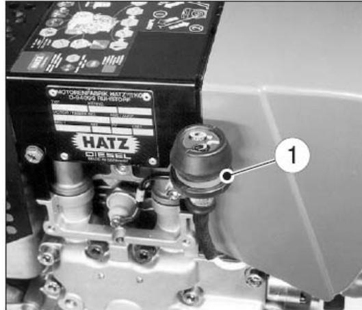
If the rubber bellow shrinks and covers the green area (Point 1), it indicates that the air cleaner system should be serviced.
