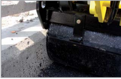
New: reduced overhang and improved wall clearance.
